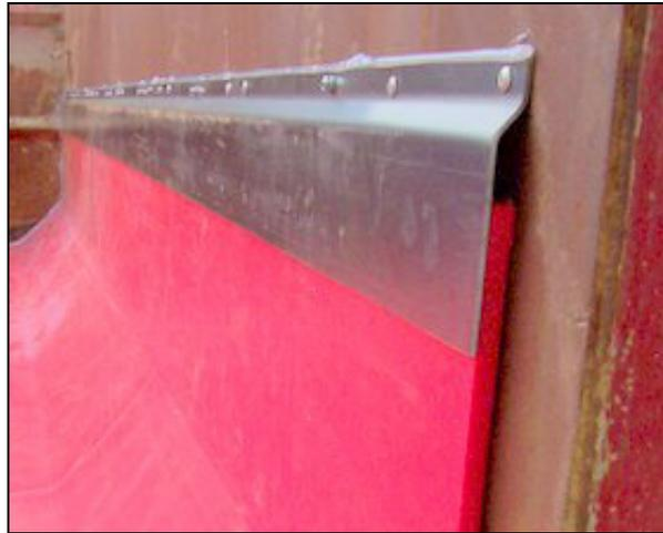
13. Fasten the cover strips by using huck rivets, welding, self-tapping screws or other fastener. It is best to stay within the support beams to conceal the fasteners on the outside of the body.
